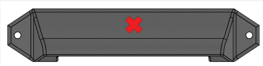
Figure 1: Wire Exit Location
