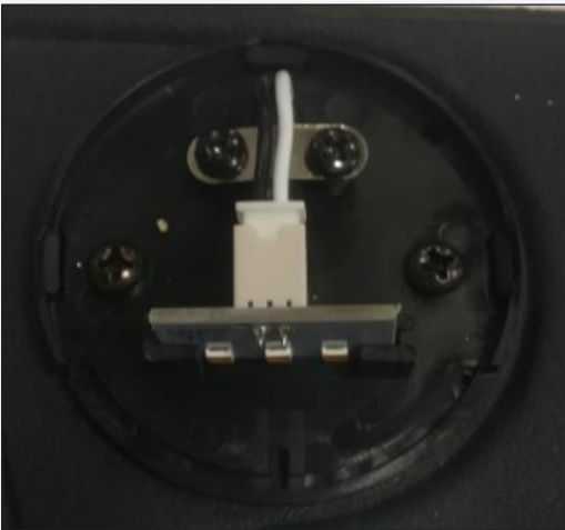
Figure 3: Base Secured with Screws
