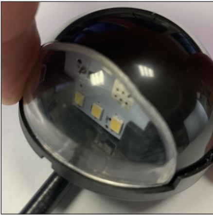
Figure 7: Insert other side of lens
