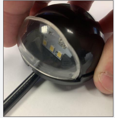
Figure 6: Insert side of lens
